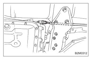
5) Connect rear oxygen sensor connector. (2200 cc)
